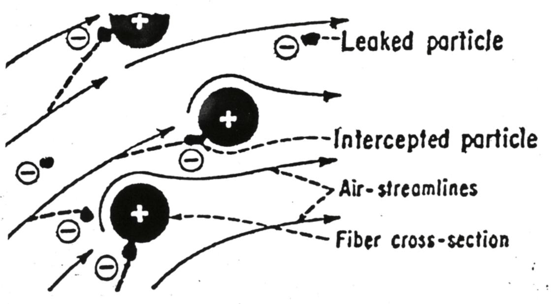
When filter fabric is charged oppositely to the dust, particles are attracted out of the air stream
